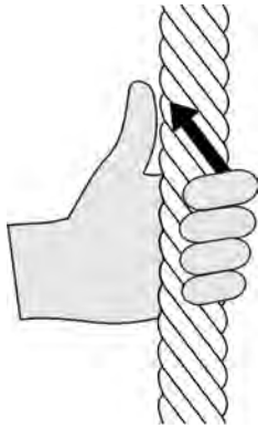
Left hand lay of strands in the rope
