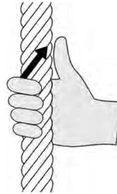
Right hand lay of strands in the rope
